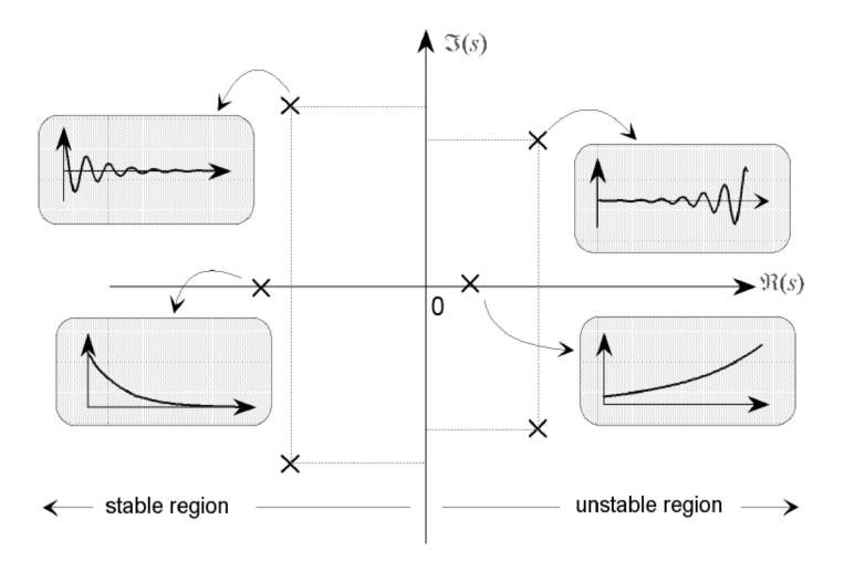
Figure 2: The specification of the form of components of the homogeneous response from the system pole locations on the pole-zero plot.
