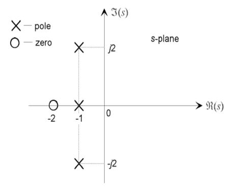
Figure 1: The pole-zero plot for a typical third-order system with one real pole and a complex conjugate pole pair, and a single real zero.
